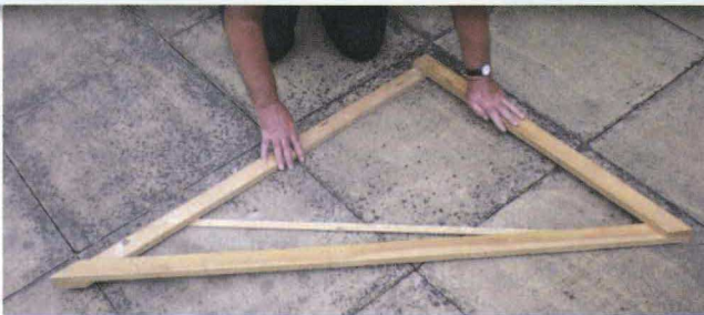
A large setsquare for setting out
