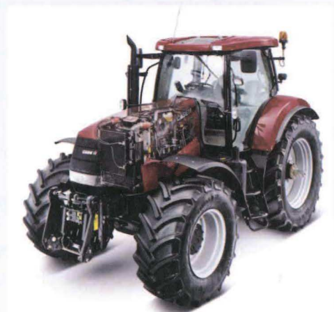
The Case-IH Puma CVX tractor is equipped with continuously variable transmission.
