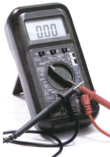
A digital multimeter can measure amperage and voltage.
